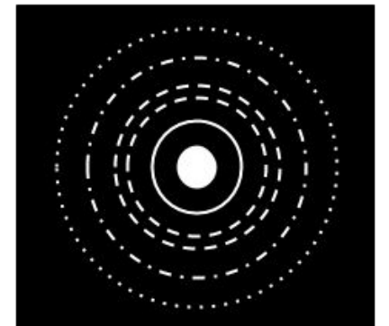
The electron diffraction interference pattern forms concentric rings
